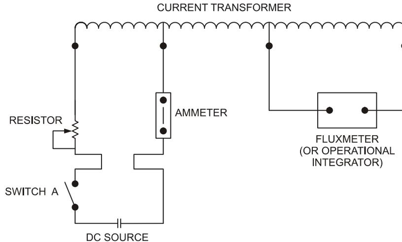
Figure 22—Method 3: Circuit for demagnetizing current transformers
