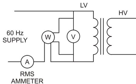
NOTE --It is recommended that the low-voltage winding be excited and the high-voltage winding be short-circuited.
