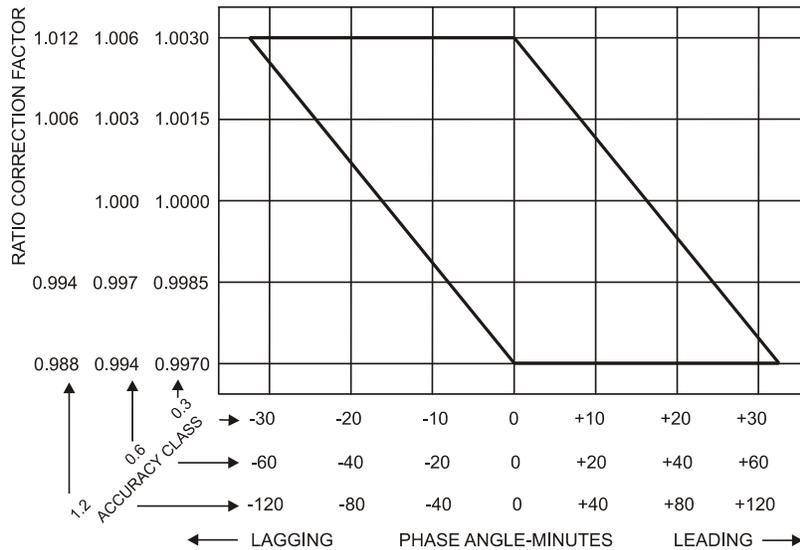
**Figure 3—Limits of accuracy classes for voltage transformers for metering**
