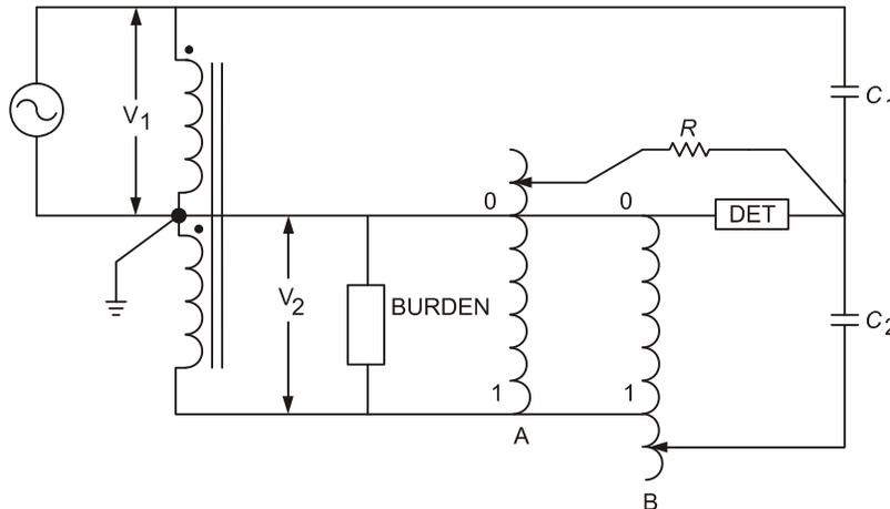
**Figure 14—Voltage transformer accuracy test (direct-null)—Capacitance divider method**
