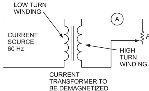
**Figure 21—Method 2: Circuit for demagnetizing current transformers**
