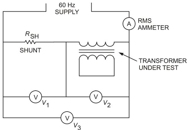
NOTE --  $V_1$  AND  $V_2$  voltmeter impedance must be high compared to shunt and transformer.
