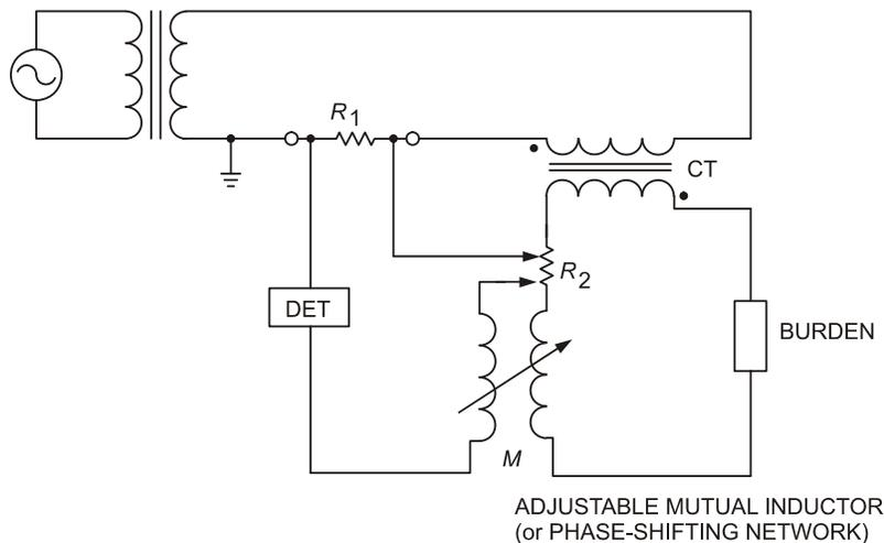
**Figure 11—Current transformer accuracy test with direct-null network**
