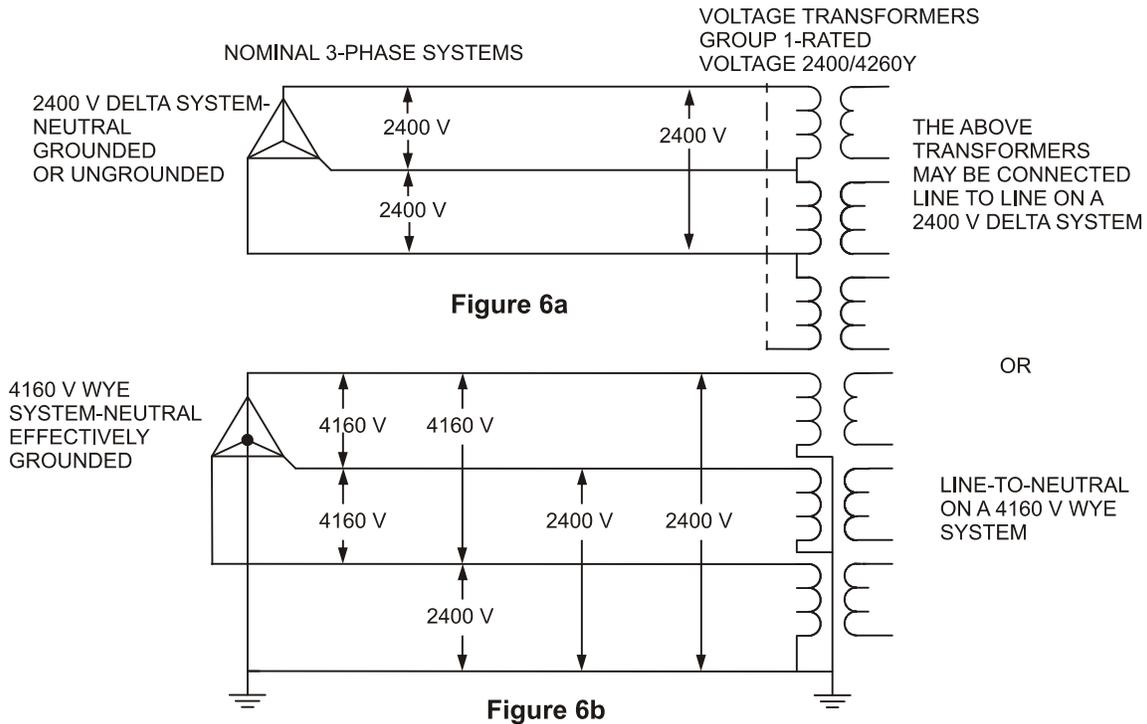
**Figure 6a and b—Typical primary connections**
