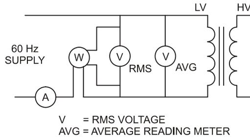
**Figure 25—Circuit for measuring excitation current and loss**
