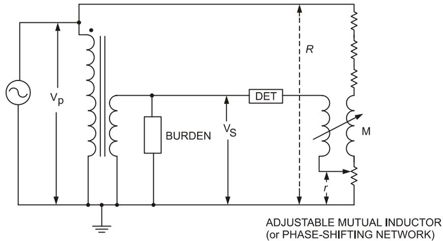
Figure 15—Voltage transformer accuracy test (direct-null)—Resistance divider method
