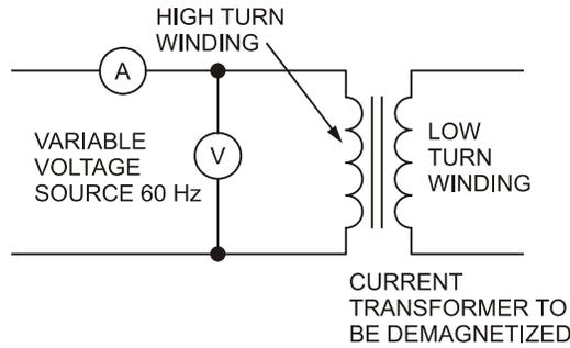
**Figure 20—Method 1: Circuit for demagnetizing current transformers**
