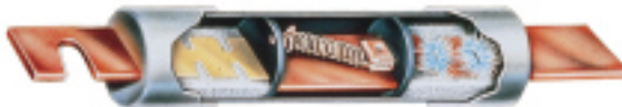
Figure 9. Like the single-element fuse, a short-circuit current causes the restricted portions of the short-circuit elements to melt and arcing to burn back the resulting gaps until the arcs are suppressed by the arc quenching material and increased arc resistance.
