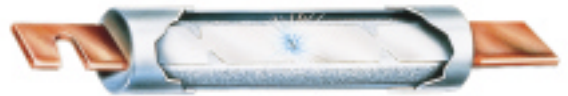
Figure 2. Under sustained overload, a section of the link melts and an arc is established.
