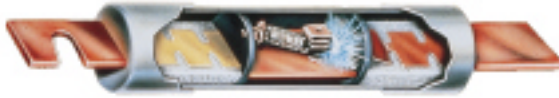
Figure 7. Under sustained overload conditions, the trigger spring fractures the calibrated fusing alloy and releases the “connector”.
