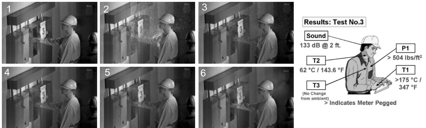
Photos and results Test 3: Staged test protected by KRP-C-601SP LOW-PEAK® current-limiting fuses (Class L). These fuses were in their current-limiting range and cleared in less than a 1/2 cycle (0.0083 seconds).
