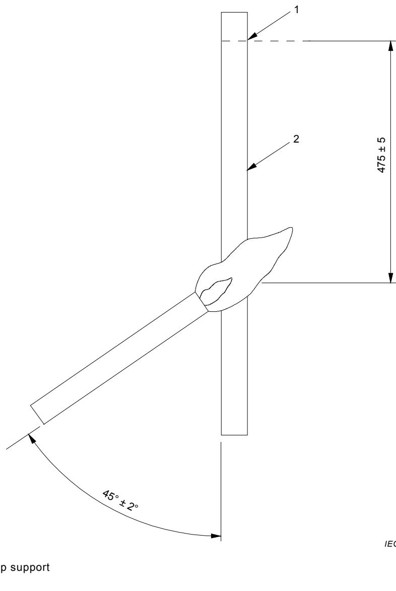
**Figure 2 – Application of flame to test piece**
