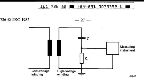
FIG. 1. — Basic measuring circuit for the partial discharge test for a single-phase transformer.
