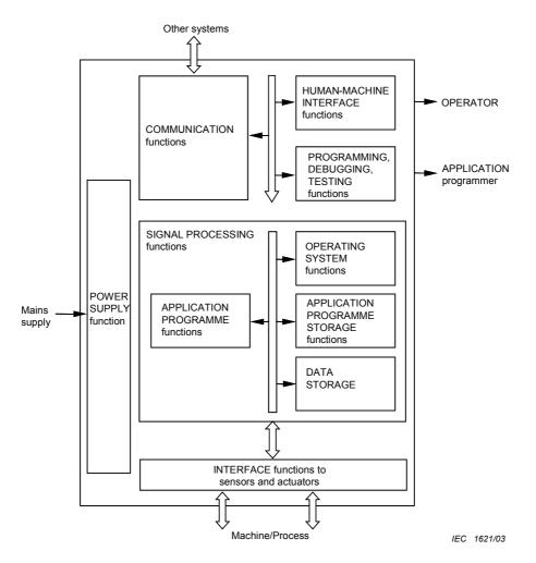
Figure 1 – Basic functional structure of a PLC-system
