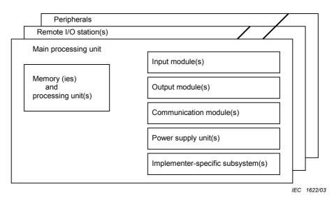
Figure 2 – Programmable controller hardware model (from IEC 61131-5)
