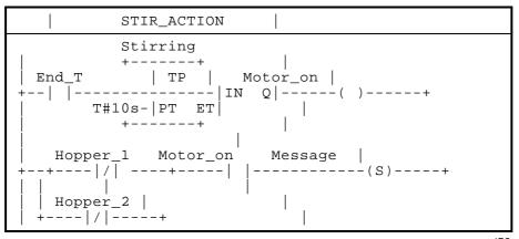
Figure 16 – Example of a programmed non-Boolean action
