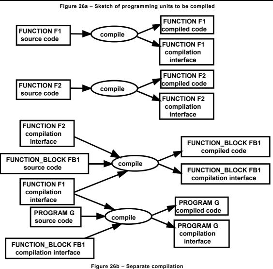
Figure 26 – Separate compilation example
