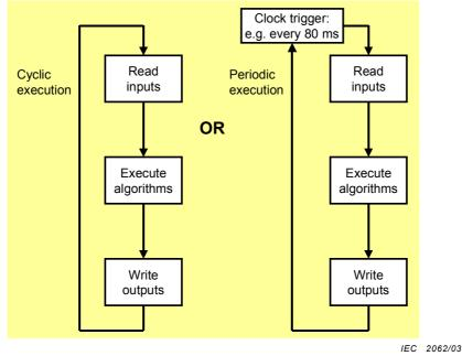
Figure 3 – Cyclic or periodic scanning of a program
