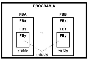
Figure 9c – Visibility of function block instances NOTE Suppression of irrelevant detail is shown by the ellipsis (...). Figure 9 – Hiding of function block instances
