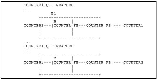
Figure 12d – Graphical passing of instance name
