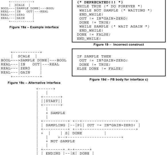
Figure 19e – Allowed SFC function block body for interface a)
