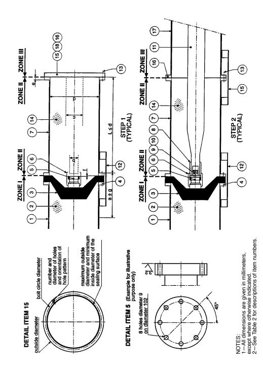
Figure 1—Typical interface drawing
