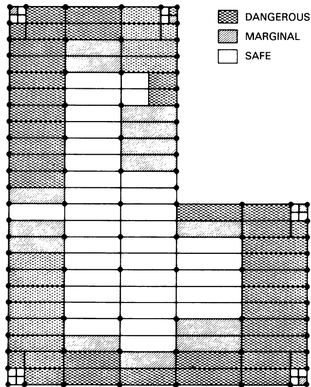
Figure 14-11—Typical ground mat design showing meshes with hazardous potentials as identified by computer analysis
