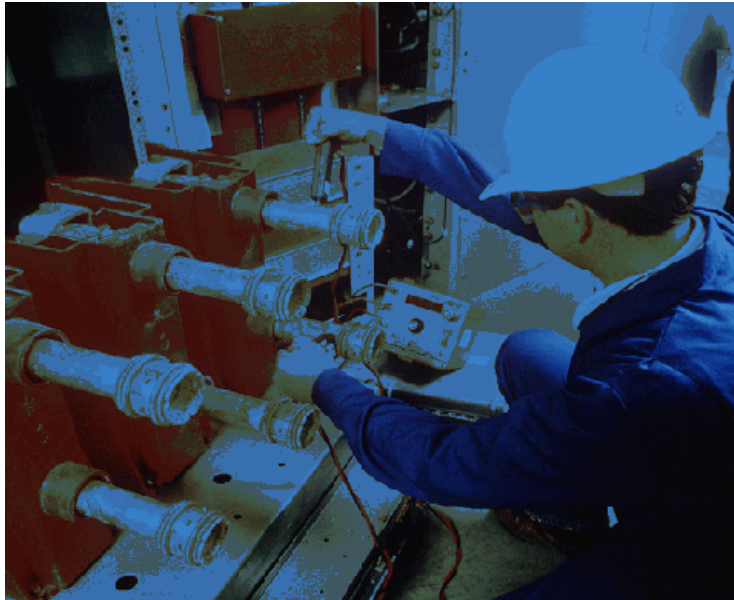
Figure 6-3—Contact resistance testing
