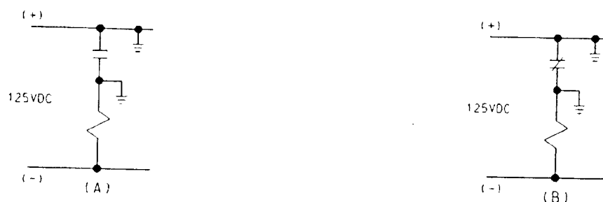
Figure C-1—Ground faults may energize a normally de-energized device or prevent de-energizing a normally energized device
