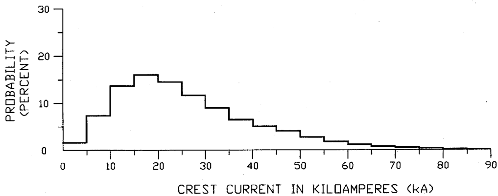
Figure 2-5 —Stroke current range probability for strokes to flat ground
