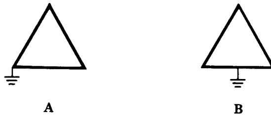
Figure 15— Grounded \Delta Secondaries A—Corner Grounded, B—Midphase Grounded
