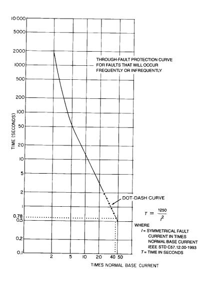
NOTE—Low current values of 3.5 and less may result from overloads rather than faults. An appropriate loading guide should be referred to for specific allowable time durations.
