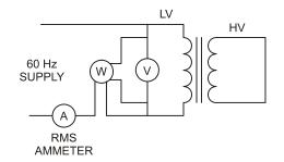
NOTE --It is recommended that the low-voltage winding be excited and the high-voltage winding be short-circuited.
