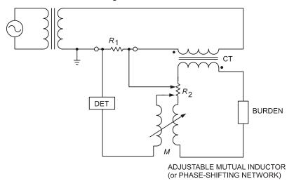
Figure 11—Current transformer accuracy test with direct-null network
