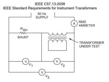
NOTE --  $V_1$  AND  $V_2$  voltmeter impedance must be high compared to shunt and transformer.
