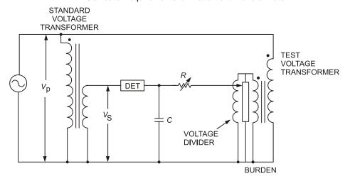
Figure 17—Voltage transformer accuracy test—Comparative-null method
