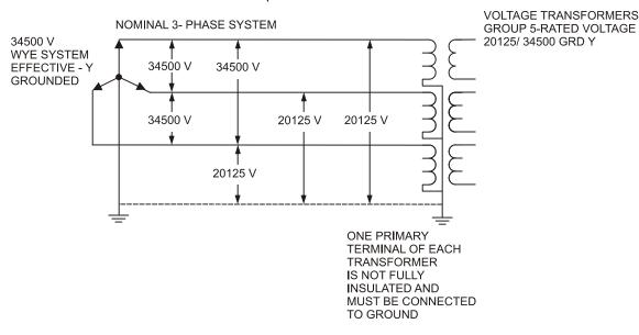
Figure 6h — Typical primary connections
