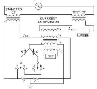
Figure 10—Current transformer accuracy test (comparative-null) composite current comparator and standard current transformer
