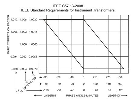
Figure 3—Limits of accuracy classes for voltage transformers for metering
