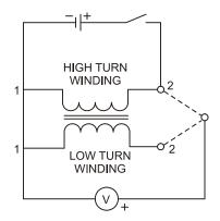
Figure 26—Polarity by inductive kick
