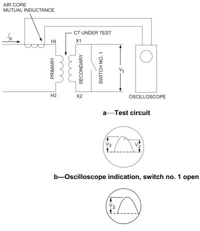
c-Oscilloscope indication, switch no. 1 closed
