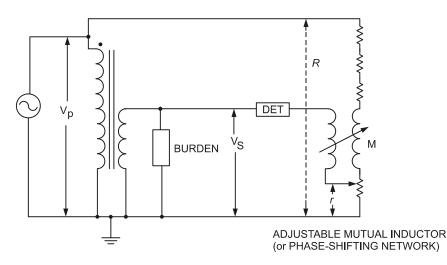
Figure 15—Voltage transformer accuracy test (direct-null)—Resistance divider method
