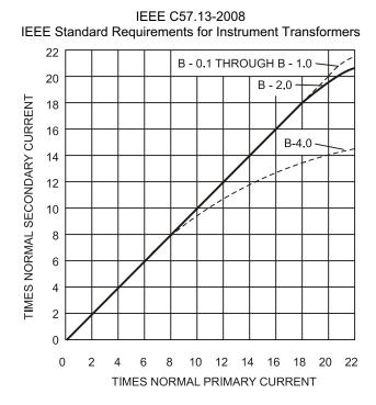
Figure 5—Typical overcurrent ratio curve
