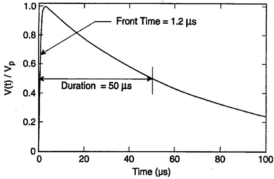
Figure 5—Combination Wave open-circuit voltage
