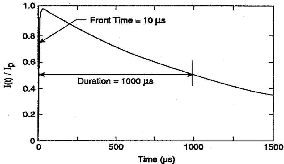
Figure 9—Waveform for the 10/1000  $\mu\text{s}$  current surge
