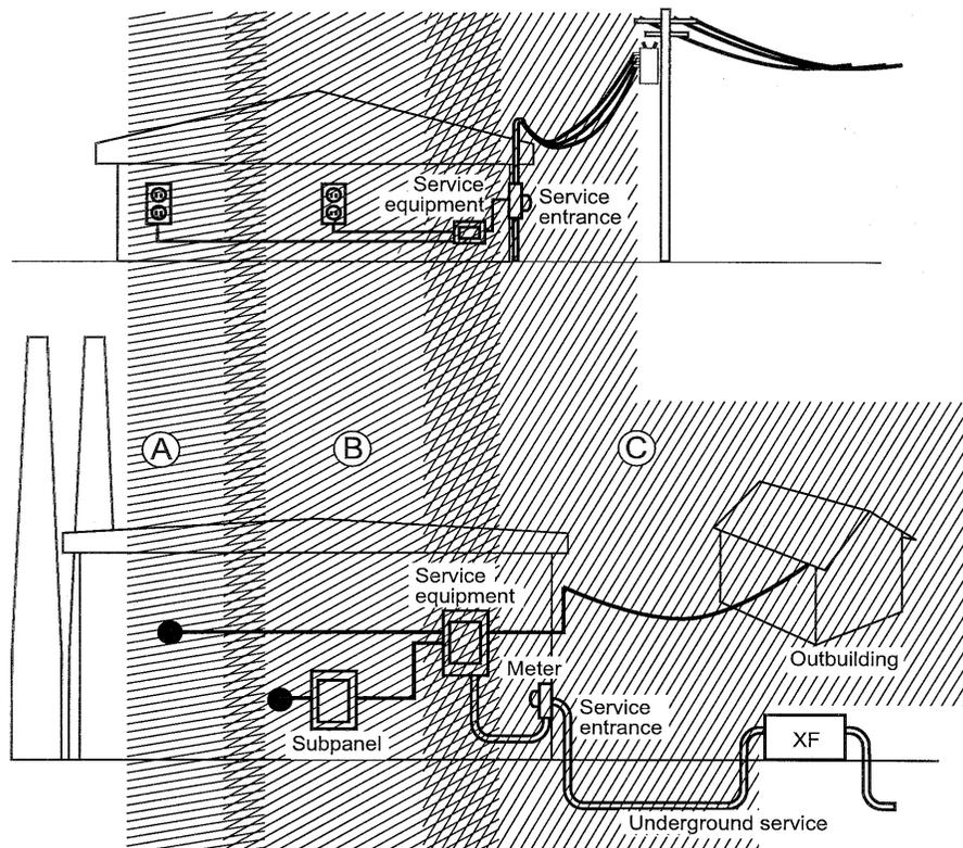
NOTE—There can be differences in the configuration and distance between the revenue meter and the service equipment. This schematic is only an example to illustrate the concept of location categories. [The National Electrical Code® (NEC®) (NFPA 70-2002) [B32] states in Article 230-70 “The service disconnecting means shall be installed at a readily accessible location either outside of a building or structure, or inside nearest point of entrance of the service conductors.”]
