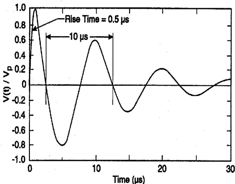
Figure 4—The 100 kHz Ring Wave (voltage and current)
