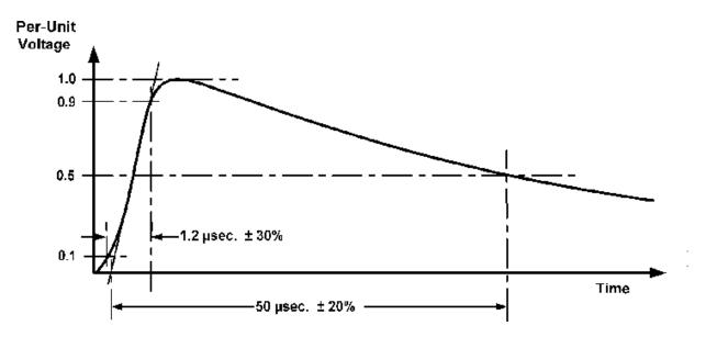
Figure 1 - Impulse Voltage Waveform
